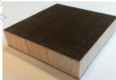
GWP production of panels with a specific rigidity of 1 kN.m<sup>2</sup>.kg<sup>-1</sup>.
